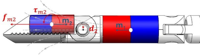
Figure S1. Static force analysis for the gripper. The gray dashed lines represent the magnetic field generated by the wrist magnet \mathbf{m}_1 . The arrow represents the field direction. \tau_{m2} and f_{m2} are the magnetic torque and force received by the jaw magnet \mathbf{m}_2 from the wrist magnet \mathbf{m}_1 which stabilizes the jaws at the closed configuration.
