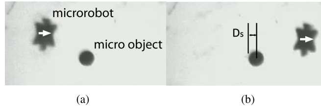
Fig. 4.1 (a) A teleoperated star-shaped microrobot and a 210\text{-}\mu\text{m} microsphere for side-pushing under liquid on a glass surface, from [154]. (b) The microrobot moves past the microsphere from its side, causing the sphere to displace a small amount D_s , primarily due to the fluid interactions. Arrow on microrobot indicates the direction of its motion.
