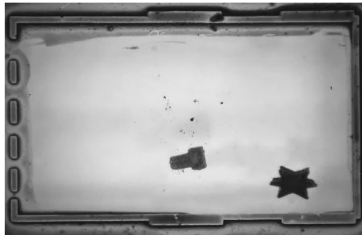
Fig. 3.3 A picture of a 500- \mu\text{m} star-shaped Mag- \mu\text{Bot} pushing a plastic peg into a gap in a 2D planar assembly task. The arena width is 4 mm.
