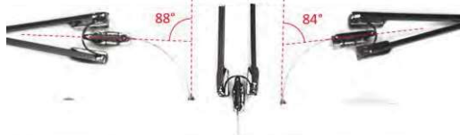
Fig. 3 (Left and right) maximum flexural wrist response to a 75 mT field oriented \pm 115^\circ away from the wrist's undeflected position. (Middle) undeflected gripper-wrist under no external magnetic field.
