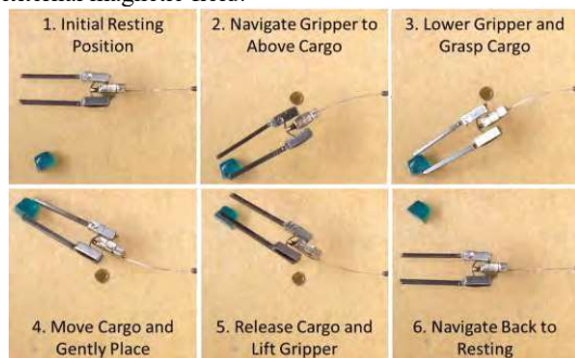
Fig. 4 Frames from the "pick and place" demonstration using the 4mm magnetically actuated gripper-wrist.
