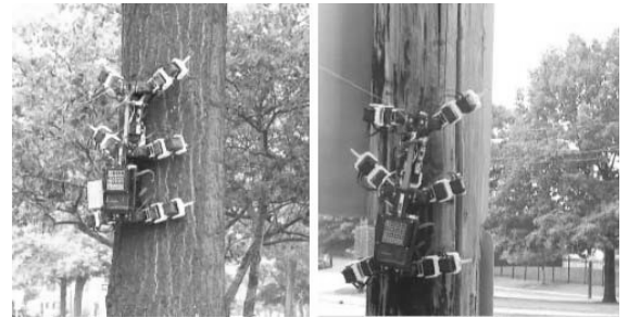
Figure 19. DIGbot climbing on a tree trunk and telephone pole with stiff claws.
