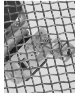
Figure 7. DIGbot claw engaged with the mesh screen.
