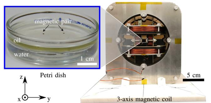
Fig. 3: Experimental setup. In the inset image of agent, two spherical microrobots sit at the interface of water-oil inside a glass Petri dish. The agents are driven in horizontal plane by an electromagnetic coil system with three pairs of coils capable of producing fields in 3D.
