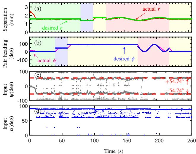
Fig. 4: (a) Separation  $r$  and (b) pair heading  $\phi$  tracking using optimization-based control at water-oil interface, (c) the in-plane control angle  $\psi$  and (d) the out-of-plane tilting control angle  $\alpha$ . RMS tracking error of less than  $50 \mu\text{m}$  and  $1.85^\circ$  is accomplished for the regulation of the separation and the pair heading angle, respectively. A video of this experiment is available as supplementary material [S1].
